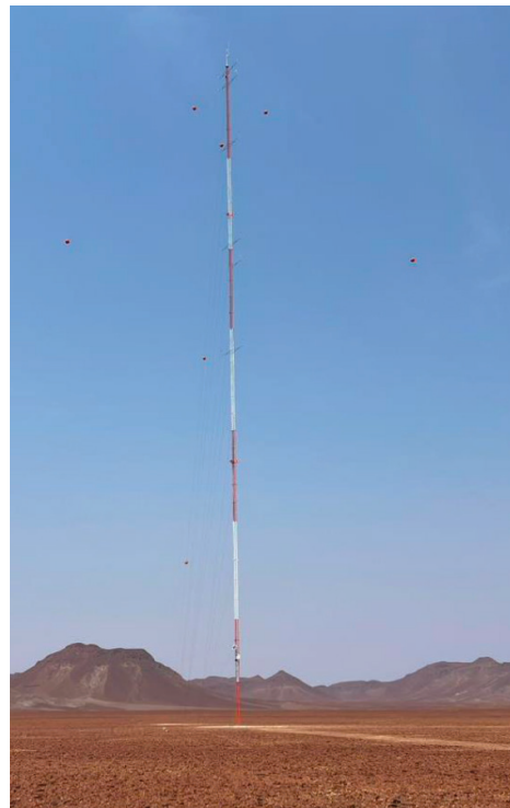
Above: MET Masts have been set up on site to record wind data at a height of 130 meters
